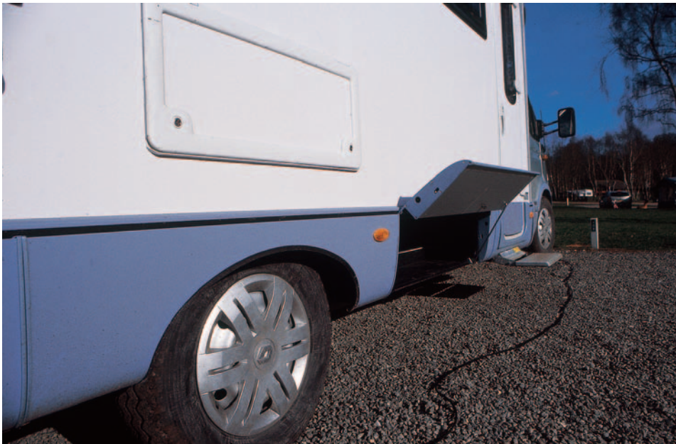
Nicely made double-skinned skirt hatches lift to reveal big storage within the double floor.
