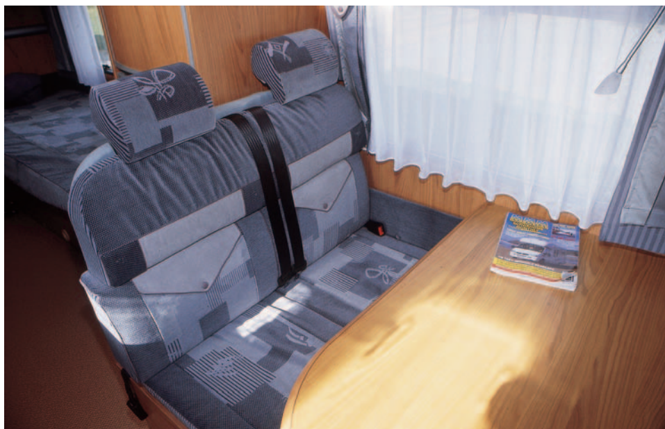
The dinette's travel seats are superb as their strong steel frame supports automotive-style, adjustable headrests.
